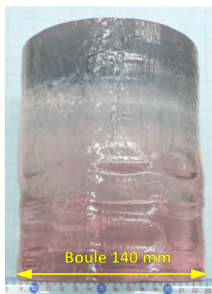
Large monocrystals developed in cooperation with Czech industry within the ELI-Beamlines project. The core-free Yb doped YAG crystals with up to 5' in diameter and 6' long are the largest of its kind in the world.
