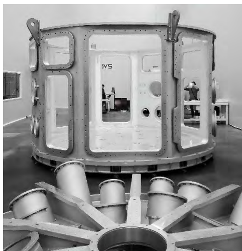
P3 Chamber: manufactured parts (left), visualization of complete chamber (right).
