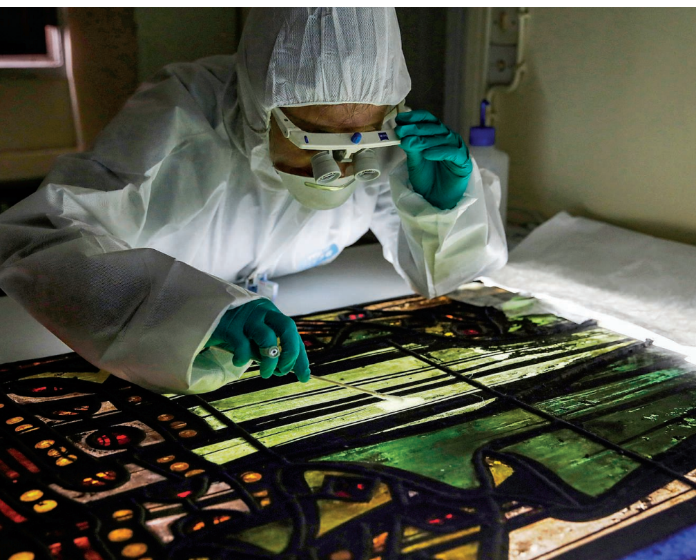
Glass researcher Claudine Loisel found that baby wipes could sample for lead without damaging staining.
